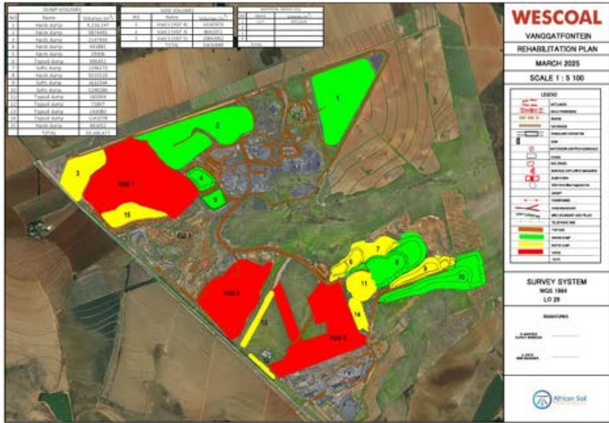
Figure 8-86. Vanggatfontein Rehabilitation plan (African Soil)
